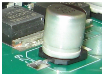
Figure 47: Wrong dimensioned electrolytic capacitor footprint
