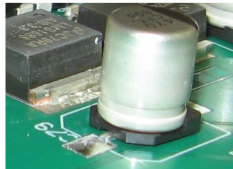
Figure 52: Wrong dimensioned electrolytic capacitor footprint
